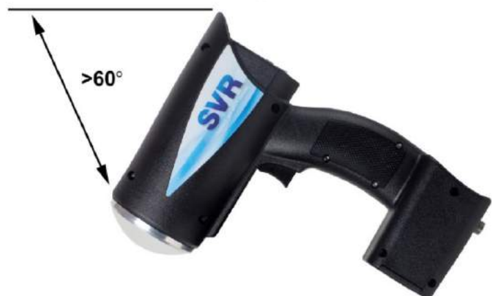
Internal cosine error correction, allowing the unit to compensate for vertical angles up to 60 degrees
